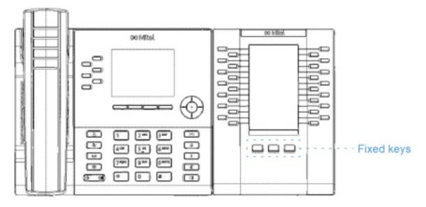
The Mitel M695 PKM features a 4.3" 480x272 pixel color backlit LCD display that provides a unified graphical user experience with the Mitel MiVoice 6920 IP phone.
