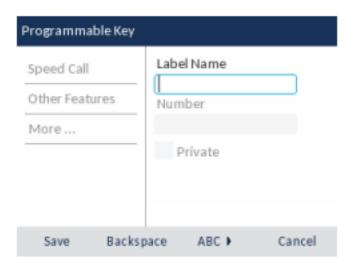
2. In the **Label Name** field, enter a label to apply to the key.
