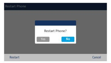
3. When the prompt, **Restart Phone?** appears, navigate to the **Yes** button and press the **Select** button or press the **Restart** softkey.
