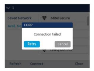
**NOTE:** If the password that you entered is incorrect, the phone normally displays the option to retry. In some cases, an incorrect password is accepted by the WLAN adapter but on reboot the Wi-Fi app auto pops up if phones fails on DHCP due to misconfiguration. You must enter the correct password again for the SSID.
