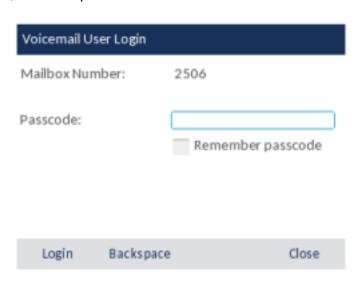
(Optional) Press the down navigation key and press the Select button to select the Remember passcode checkbox.
