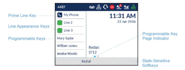
If you have six or more programmable keys configured, programmable page indicators are displayed above the softkeys. These dots indicate the number of programmable key pages and its relative position. Press the left and right navigation keys to switch the programmable key pages.
