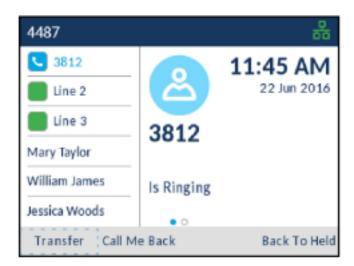
4. Press the **Transfer** softkey or hang up the handset to complete an unattended call transfer
