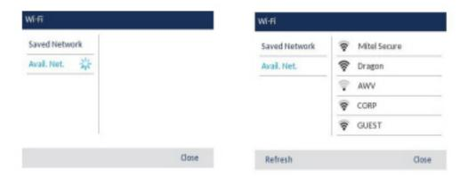
4. Select an SSID (that is, the name of a Wi-Fi network, for example, **Mitel Secure**) from **Avail. Net** (Available Networks) to connect. If the SSID is secured, a password prompt appears.
