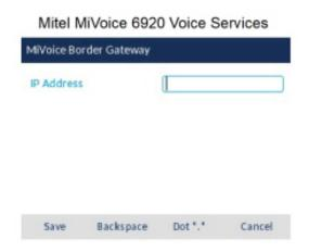
**NOTE:** The **Backspace** softkey can be used to delete the last digit/character entered and the dot (".") softkey can be used to enter a dot where applicable.
