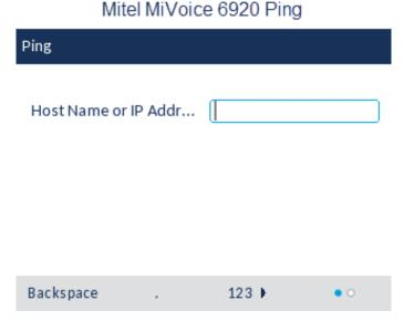
3. In the input field, enter the host name or IP address of the network endpoint you want to ping using the dialpad keys.
