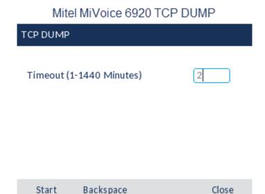
3. In the **Timeout** input field, enter the amount of time (in minutes from 1 to 1440) you would like to capture TCP network packet data using the dialpad keys.
