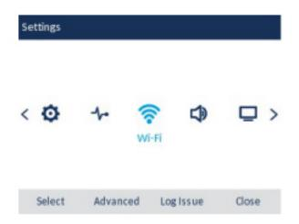
2. Ensure that a WLAN adapter connected to the phone. The phone displays an error if it is not connected to a WLAN adapter.
