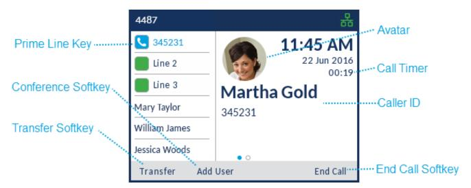
Additionally, if the call is on the **Prime Line** key, the **Prime Line** key changes to reflect the status of the line as per the following table.
